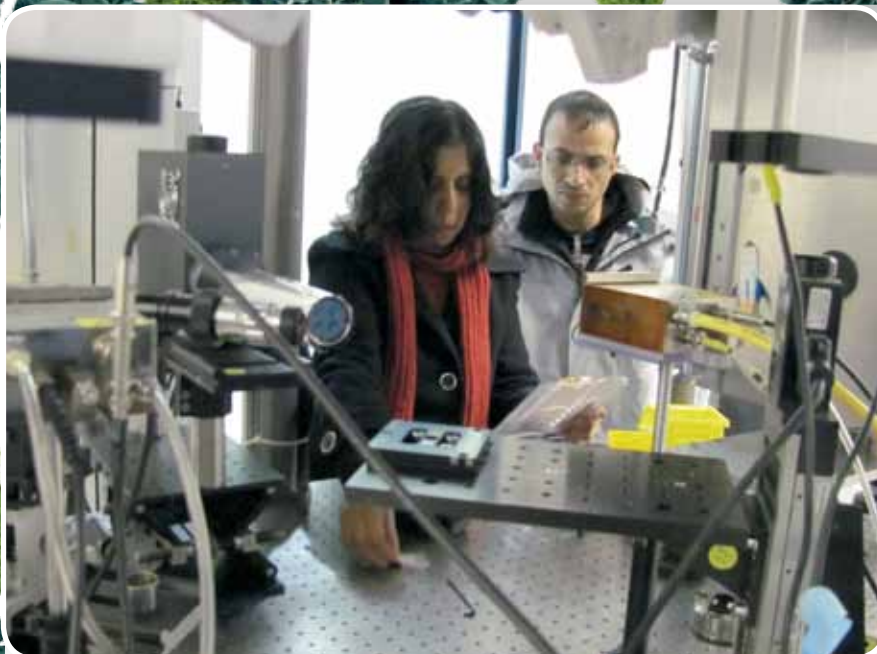
Ganga Hettiarachchi, Kansas State University, shows graduate student Raju Khatiwada how to mount the sample holder with soil samples on the xyz stage of a beamline at the Advanced Photon Source, a national synchrotron X-ray research facility at the Argonne National Laboratory.
